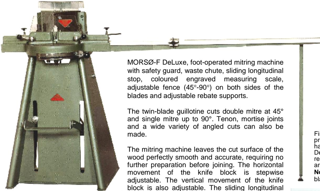
MORSØ-F DeLuxe, foot-operated mitring machine with safety guard, waste chute, sliding longitudinal stop, coloured engraved measuring scale, adjustable fence (45°-90°) on both sides of the blades and adjustable rebate supports.
