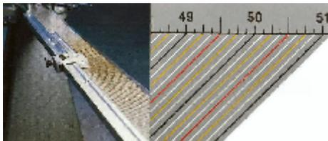
Precision engraved measuring scale is now standard on the DeLuxe mitring machines. The lines are colour coded for enhanced discrimination and size setting.
